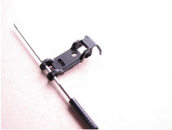
Opening out to 2mm with a cutting broach.
