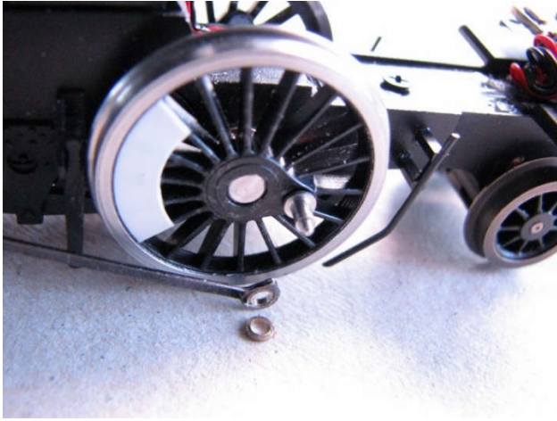
Washer placed on crankpin before the rod.
