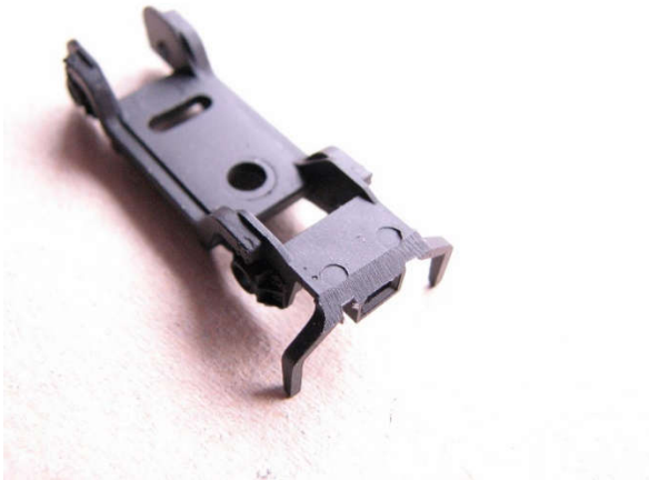
Bogie front upper leading edge chamfered.
