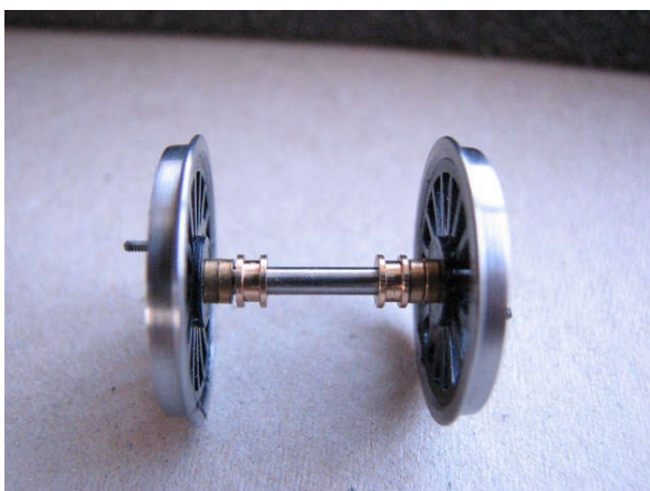
Wheels and bushes assembled on an axle.
