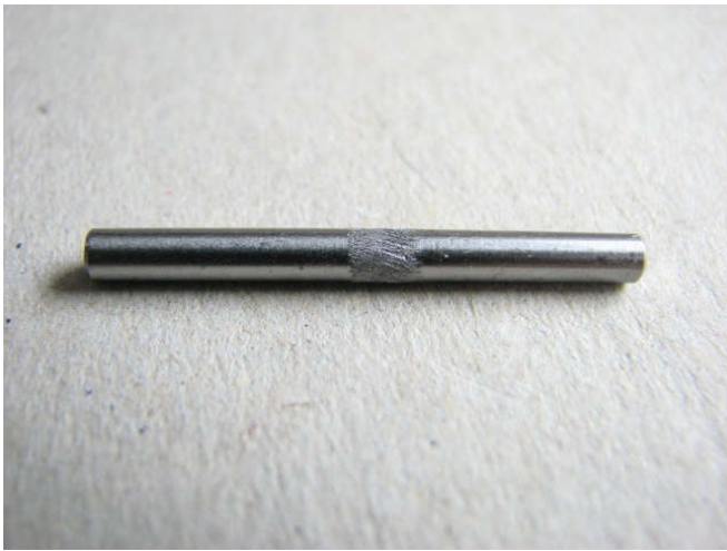
Axle knurled for gear.
