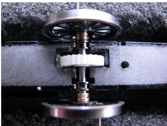
Driven axle with spacing washers placed in chassis.
