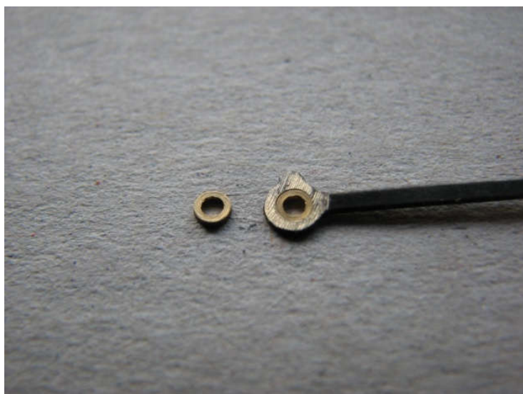
Bush inserted into rod ready for soldering.
