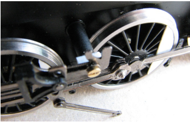
Packing inserted behind radius rod and new 12BA screw.
