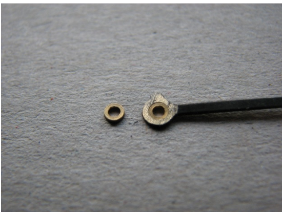
Bush inserted into rod ready for soldering.
