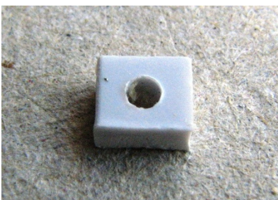
60 thou packing piece, 3mm x 4mm, with a 12BA clearance hole.
