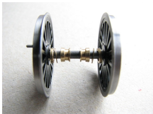
Leading wheelset with spacing washers and bushes.
