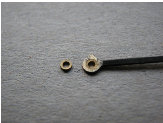
Bush inserted into rod ready for soldering.
