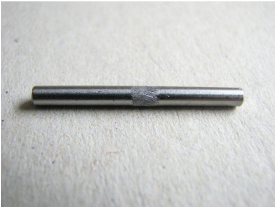
Axle knurled for gear.
