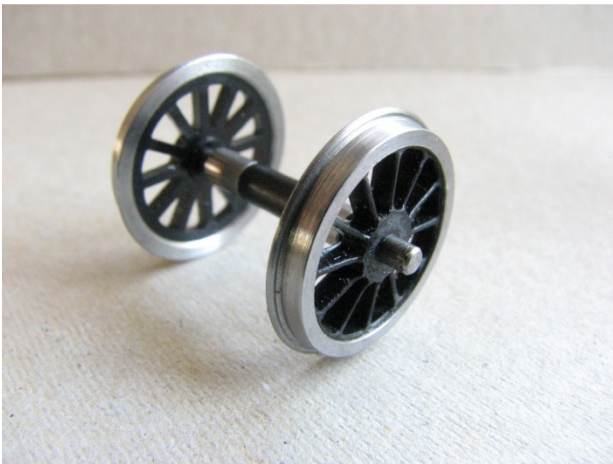
Gibson wheels mounted onto Bachmann axle.
