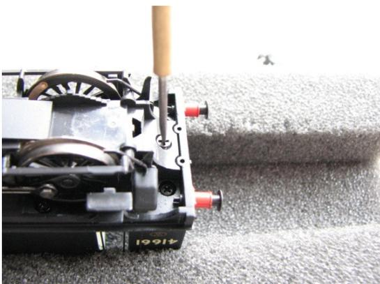
Undoing body retaining screws.
