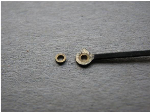
Bush inserted into rod ready for soldering.
