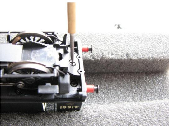
Undoing body retaining screws.
